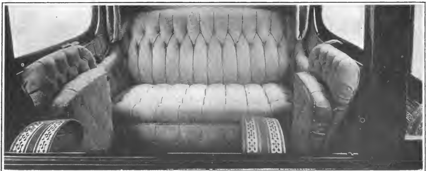
Fig. 3—View of the interior of the limousine, showing the upholstery and extra seats folded away
